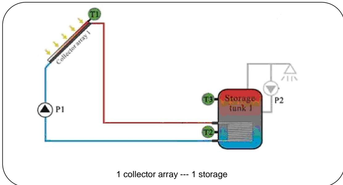
T1: Temperature sensor for collector array
