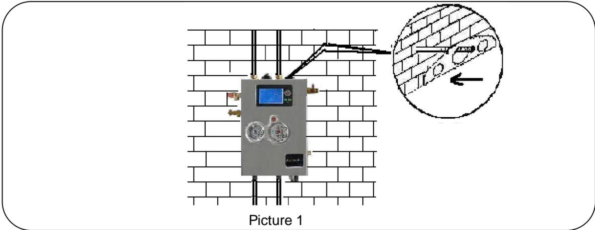
2. Drill the holes for dowels, put the dowels into the holes, fixed the solar control system on the wall using fastening screws. The solar control system must be vertically installed. See picture 2.
