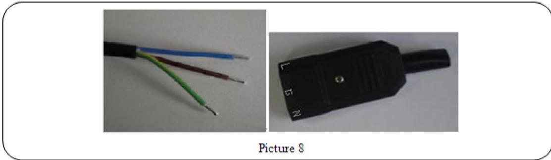
3. To connect external circulation pumps or any electromagnetic valves, firstly loose the aviation socket and dismount it as indicated below. Connect the wire to aviation socket, number 1 connects “N” wire (blue color), number 2 connects ground wire (yellow-green color), number 3 connects “L” wire (red color). Reassemble the aviation socket and connect it to the solar control system.
