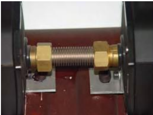
Two collector headers joined.
